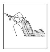
If the position you are using has an adjustable headrest or head restraint and you are using a dual tether, route the tether around the headrest or head restraint. 3. Push and pull the child restraint in different directions to be sure it is secure.
